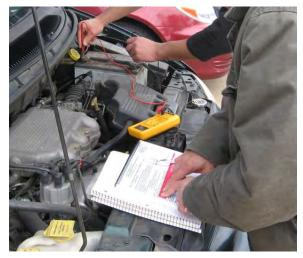
Technicians are going through *FIRST THINGS FIRST* for the first time. Each test step is fully explained on the left side of the page and an illustration of the DMM test leads connected to the vehicle is shown on the right side of the page for added clarity. These tests will reveal a weak or undercharged battery, a faulty engine or accessory (sheet metal) ground circuit, and a poor performing charging system.
